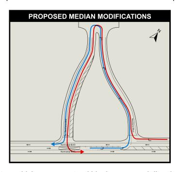
This rendering illustrates vehicle movements within the proposed directional median. To enhance safety and traffic flow, delineators will be installed to prevent westbound left-in movements from obstructing the through lane and adjacent left-turn lane. These delineators will also restrict direct left-out movements from the development. However, all restricted movements will continue to be accommodated via the developer's internal roadway network.
